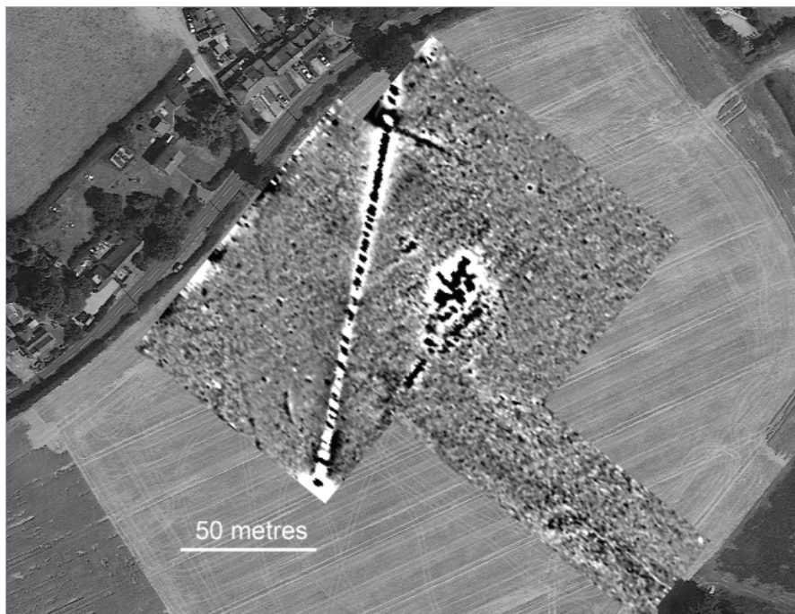
Figure 1: Magnetometer survey of the Guestling Thorn bloomery; the diagonal line is a modern feature (David Staveley)
