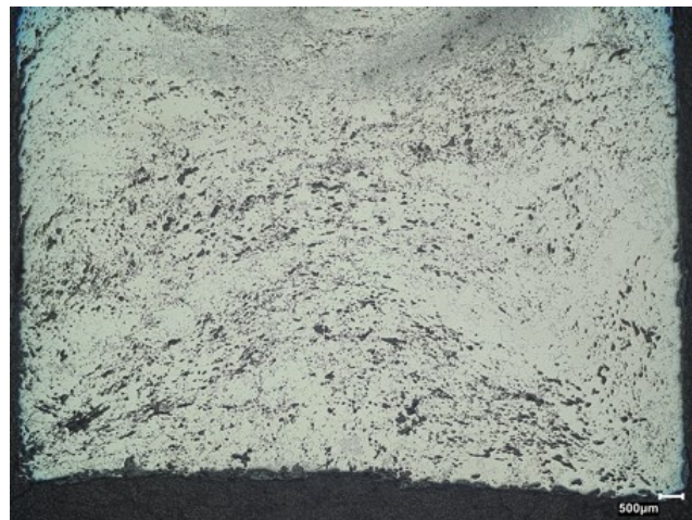
Fig 3. Cross section of a nail from the Weald c 1650. Note the enormous amount of slag and the dark areas of high carbon content.
