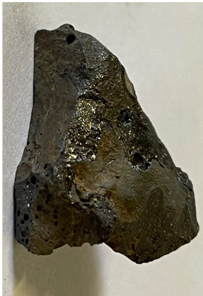
Fig. 2. Part-ground part of specimen shown in Fig. 1. Shiny flakes of iron visible.
