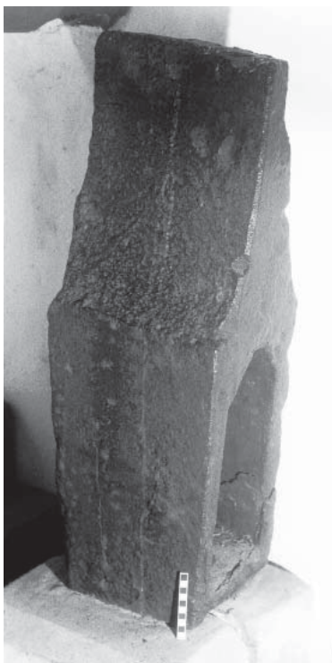
Figure 2: Cast-iron forge hammer from Etchingham Forge (scale 10cm); Anne of Cleves House, Lewes, Sussex.
