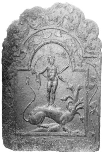
Figure 1: Wooden pattern for a fireback from Ashburnham Furnace, showing Hercules fighting the Hydra; Anne of Cleves House, Lewes Sussex
