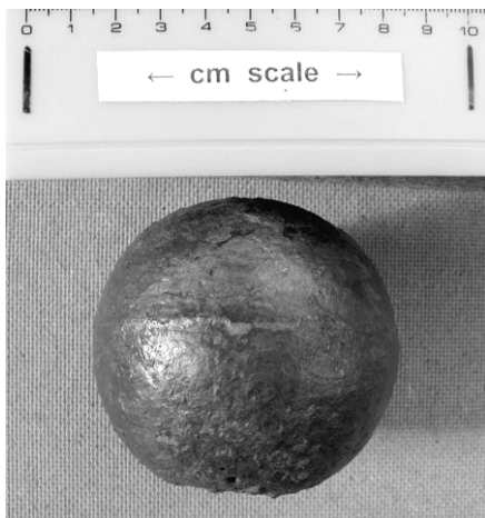
Figure 2 – Cannon proofing ball approx. 81mm (3.18 ins.) weight, approx. 2.1kg (4lb 10oz)
