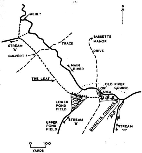
FIG. I. THE LEAT FOR AVERIES MILL AND BASSETTS FURNACE
