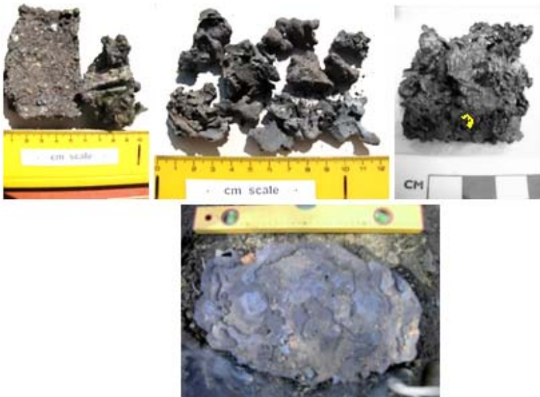
Figure 1 – L to R: Furnace, Cinder, Bloom & Tap Slags
