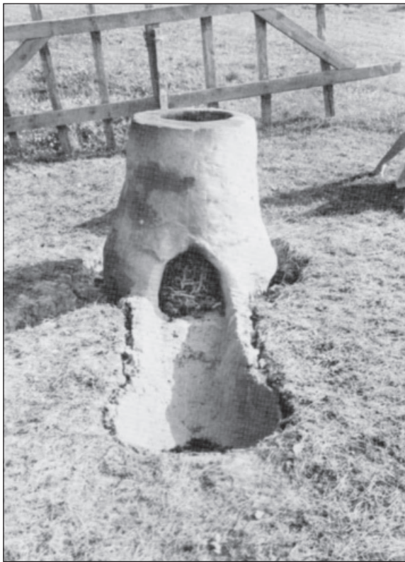
Fig 5: The original 2ft 6in experimental furnace preparatory to drying.
