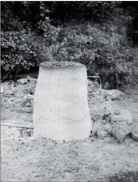
Fig 9: The furnace as enlarged, showing thermocouples. (T1 is not visible)
