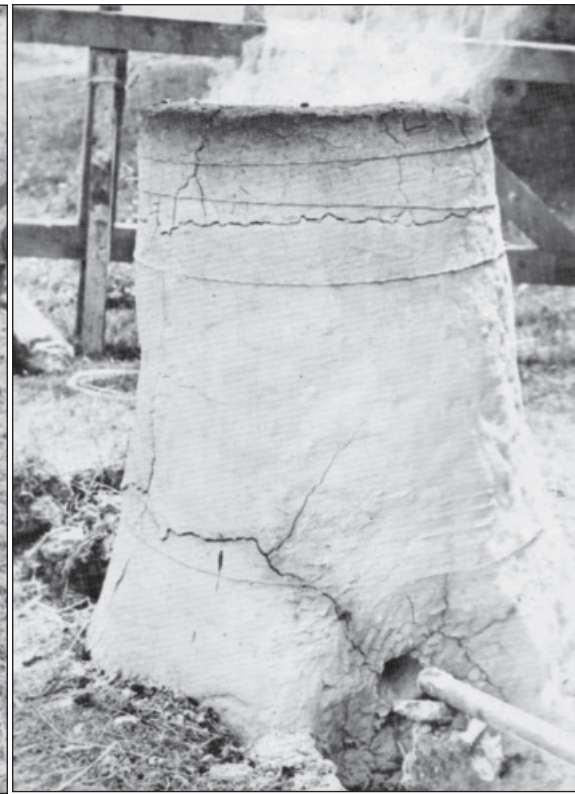
Fig 6: The enlarged experimental furnace showing method of stopping up the furnace arch
