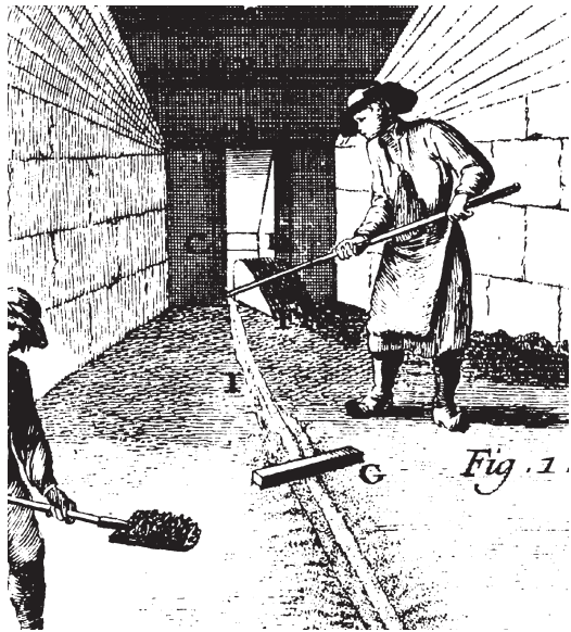
Figure 4: Illustration showing the flow of iron from the forehearth past the damstone, along a runner into the pig bed (from Diderot & Alembert, Encyclopédie, 1762)
