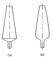
Fig. 3: The original discontinuous Walloon shaft profile (a) and a more rounded (German) version (b)
