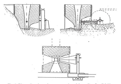
Fig. 4: Plan and sections of a reconstruction of the earliest Swedish blast furnace
