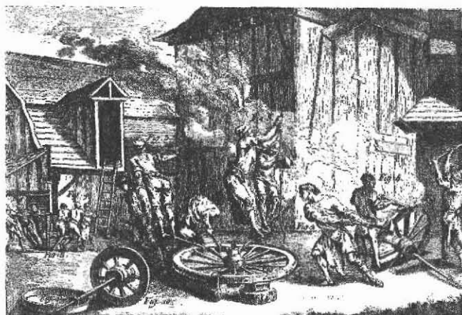
A wheel being tyred - Plate 175 from Diderot
