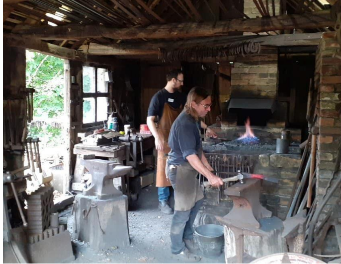
Figure 4.83 - Secondary smithing taking place at a smithing hearth within a blacksmiths shop. (Author's image).
