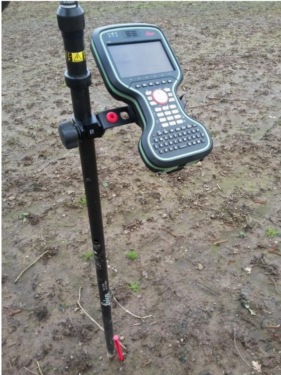
Figure 4.1 – Leica GPS positioner. A pre-planned grid meant that a highly accurate grid of 20m x 20m squares could be plotted across the field and marked with red tent pegs. (Author's image).
