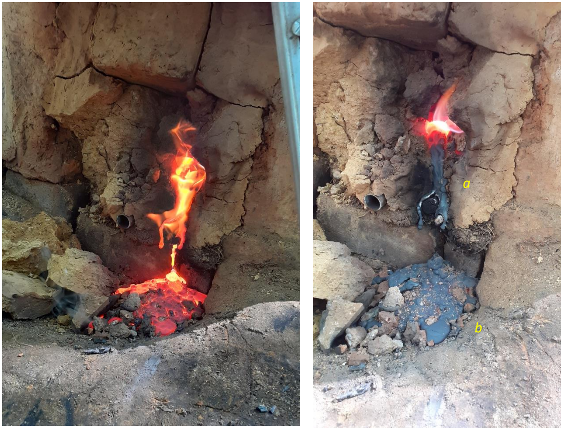
Figure 4.87 - Runs of tap slag are released, in some cases solidifying as vertical flows (a), while others amalgamate in the tapping pit (b) (see below). Further flows accumulate in the pit leading to the formation of slag cakes demonstrating layers of flows. The morphology of type 2 slag at Roffey suggest these were removed during the smelt. However, at Tudeley flows of tap slag were allowed to build up into thick cakes, possibly over several consecutive smelts. Refractory material from the tapping arch adhere to the base of the slag. Some slag solidifies in the hole left by the boring stick to create Type 3 rod slag. (Author's image).
