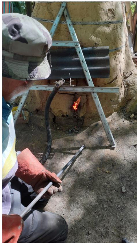
Figure 5.69 – use of a boring stick at the Pippingford experimental smelt and the release of heat and light. (Author’s image).
