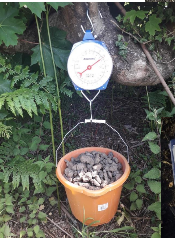
Figure 4.17 (above) – The slag from each grid, having been sorted into size groups was counted and weighed before a sub-sample was saved. (Author’s image).
