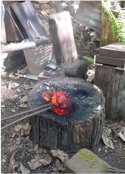
Figure 4.95 - The bloom is consolidated, and slag is driven off and build up within the hearth to form consolidation slag or primary smithing slag. This was recorded as Type 1 (WR) (right) at Roffey and constituted 6.10% of the assemblage. (Author's image).
