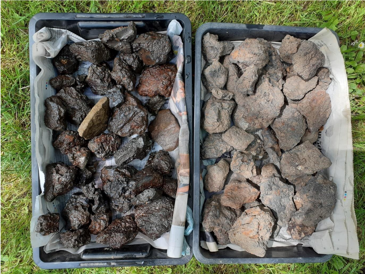
Figure 4.30 - Recently washed slag compared to washed and dried slag. It was apparent during the washing process that wet slag was often easier to determine the morphological characteristics, such as colour and inclusions. While it was impractical to analyse the slag while wet, an adapted methodology could consider this in future projects. During the original collection of the slag, on wet days the slag stood out more clearly against the soil than on bright sunny and dry days. (Author's image).
