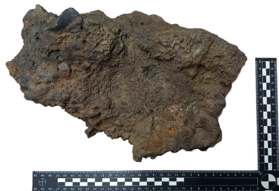
Figure 3.88 – Image of large slag found at Brook Lane. Concave convex in shape with some traces on tendrils and rust deposits. High density, weighing 4800g. (Author's image).
