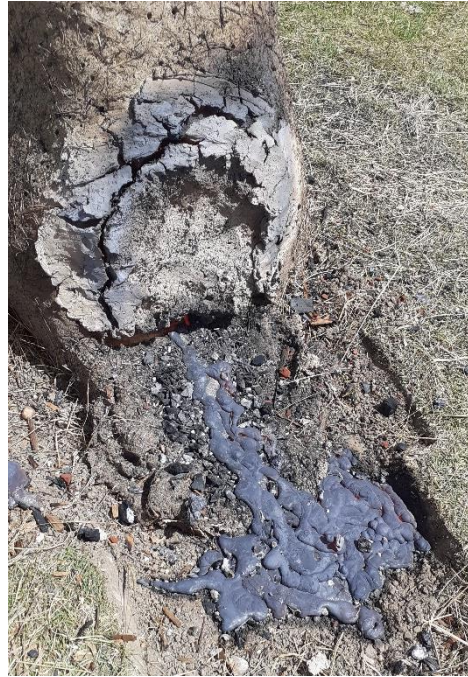
Figure 4.79 - Solidified Tap slag having flowed from a gap underneath the blocked tapping arch. This was classified as Type 2 in the Roffey assemblage. (Author's image).
