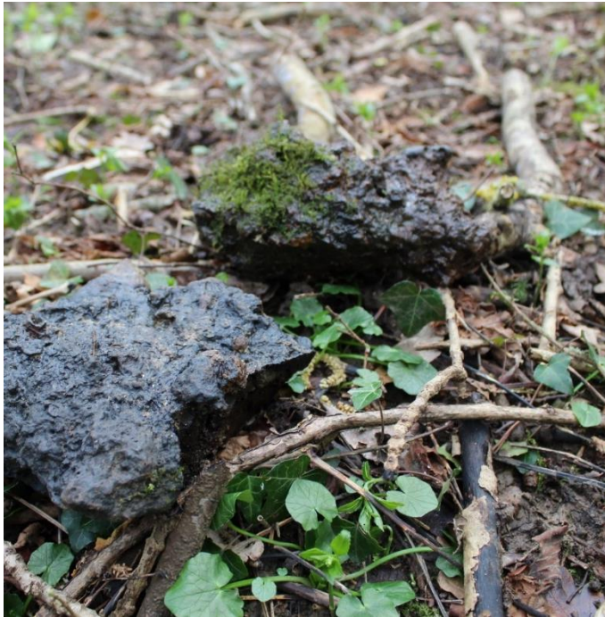
Figure 2.3 – Examples of Wealden slag typically recovered on a foray from a stream channel (Authors image)
