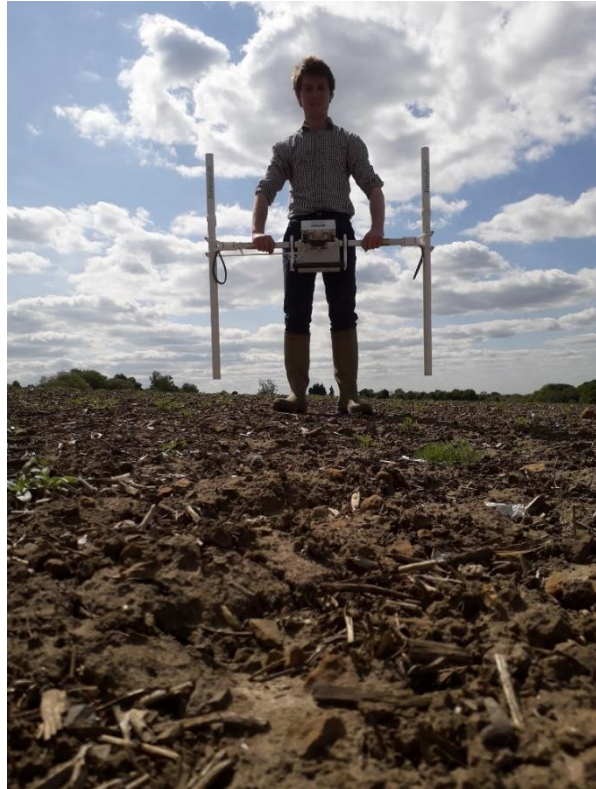
Figure 2.12 - Bartington Fluxgate Gradiometer Grad601r in action at Roffey. (Authors image)
