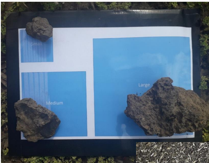
Figure 4.14 (left) – Using a standardised size chart, slag was sorted into size categories and each category was counted, weighed and photographed. (Author’s image).
