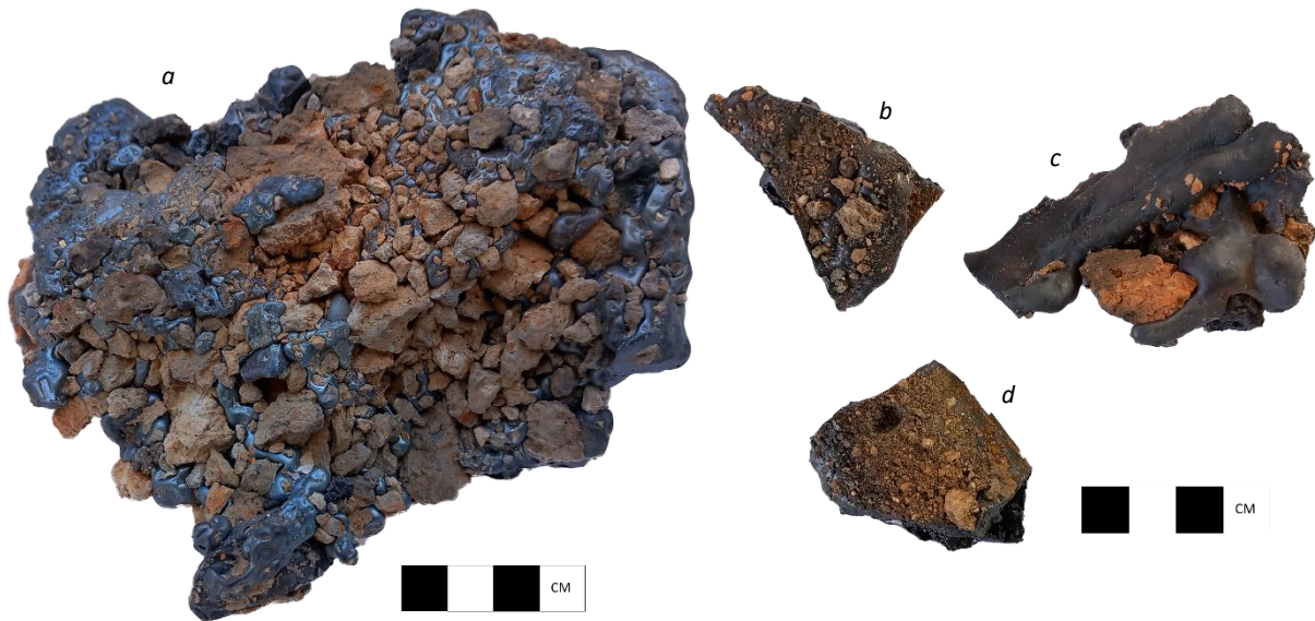
Figure 4.93 - Tap slag with refractory material from the tapping arch adhering to the underside (a). It can be seen how the slag has a smooth undulated texture which parallels examples from Roffey (below). B and d show evidence of soil adhering to the underside which was also seen as impressions in Type 2 and 4 slag at Roffey, the soil presumably wearing away over time. (Author's image).
