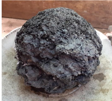
Figure 4.77 - Iron bloom from an experimental smelt at Pippingford. The bloom still retains a lot of slag and must be further refined before the iron can be utilised. (Author's image).
