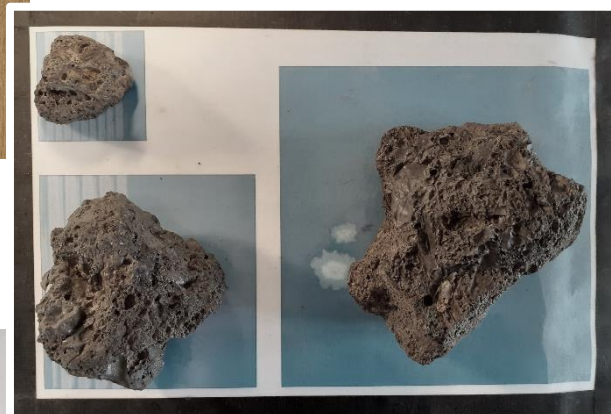
Figure 4.40 (left) - Photographs of each individual slag and geology type were also made to record a higher degree of morphological detail that would not be visible in the larger photograph. A photographic record of each assemblage of slag and geological material was also created for future interpretation and cross examination of slag types. (Author's image).
