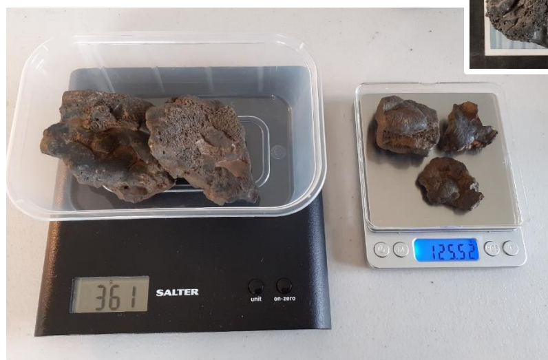
Figure 3.42 (left) – all samples were weighed initially as a total of the overall grid / transect stint, then by their individual size groups and finally examples of the small, medium, and largest within each. (Author's image).
