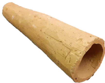
Figure 4.76 - Left a tuyere embedded in the wall of an experimental bloomery furnace. Right, a Sri Lankan tuyere made of fired clay. The Tudeley accounts record how the tuyeres were made of iron. (Author's images).
