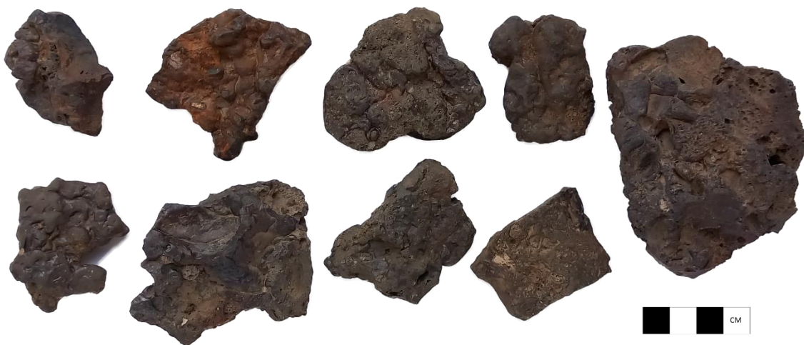
Figure 4.94 - The underside of tap slag examples from Roffey. The smooth undulated texture parallels the experimental samples above and indicates that in the same way this slag once had refractory material adhering to its underside. 25.5% of the Roffey Type 2 assemblage had refractory inclusions remaining within the slag, while other inclusions such as ore also dominated (31.4%). (Author's image).
