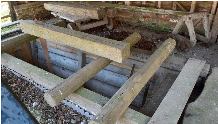
Figure 6.26 – Reconstructed sawpit at the Weald and Downland Living Museum. The sides of the pit in this instance were boarded, while above the pit stood a frame to support the timber. (Author's image).
