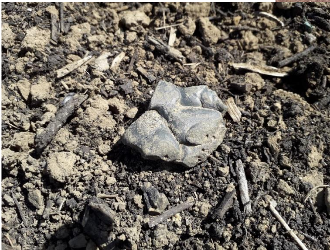
Figure 4.12 (left) – One of the many fragments of tap slag collected during fieldwalking. The majority were small and heavily fractured from their time in the plough soil. (Author's image).
