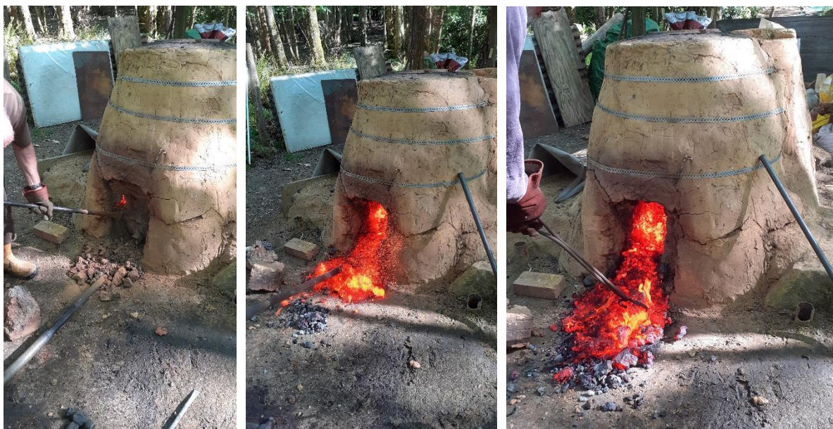
Figure 4.90 - The boring stick was used to fully open the tapping arch which released mixtures of unburnt charcoal and amorphous slag, at Roffey classified as Type 1. (Author's image).
