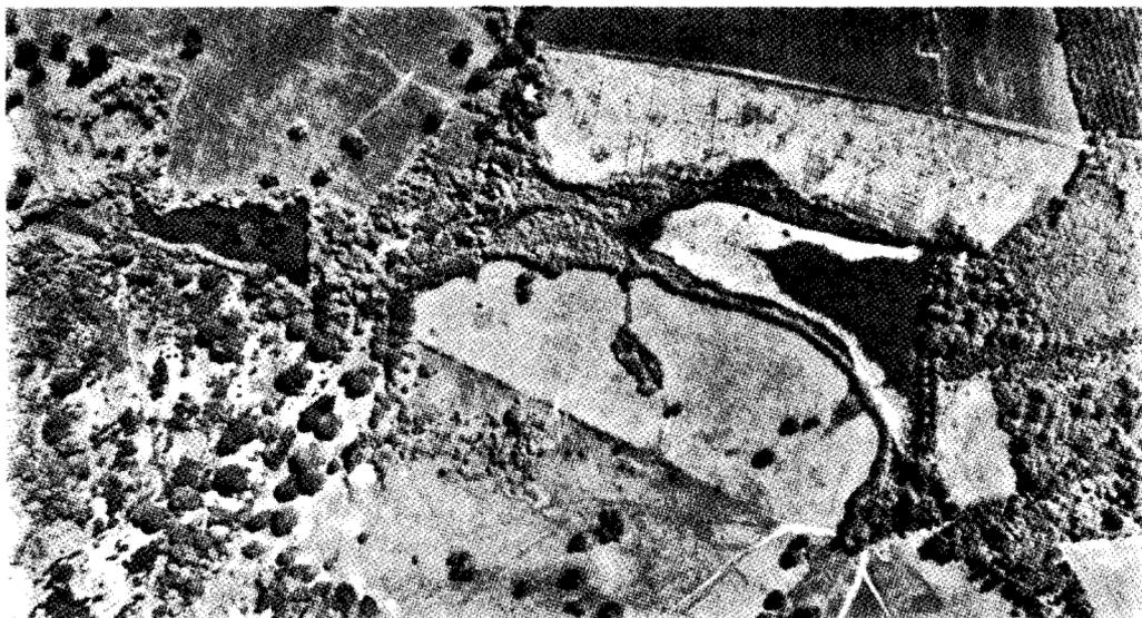
Fig.47 Eridge furnace (TQ 564350). This vertical air photograph illustrates a system of pen ponds frequently used by Wealden ironmasters. The furnace lay in the wood to the right, close to the bay. The main pond, with weed and silt diminishing its size, has a spillway at each end, one being clearly visible. Two pen ponds can be seen towards the left of the picture (Cambridge University Collection: Crown Copyright reserved).
