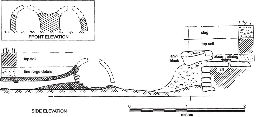
*Fig 4: Sections of furnace*
